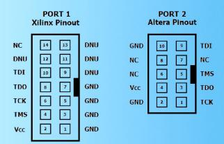
TDI - Data to device TDO - Data from device TCK - Clock signal
