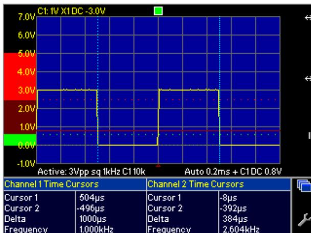
◀ Here, with the same thresholds, is a 3V logic signal. You can clearly see that this signal is still valid with our threshold settings. In a circuit with 3V and 5V logic standards, this signal would be compatible with both standards and may well be found in the interface between the two types of logic ICs on your board.
