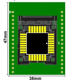
Pin 1 of the DIP base, and Pin 1 of the Device are both marked on the PCB, as per the above image
