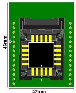
Pin 1 of the DIP base, and Pin 1 of the Device are both marked on the PCB, as per the above image
